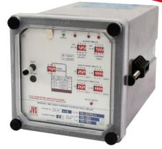
The relay measures the line current from each of the phases and if exceeds the set operating current, then relay extends a trip signal after the operating time. The relays operating time is determined by selecting one of the four inverse time current characteristics. The relay has facility to active / inhibit the high set protection feature. The relay output contacts are self reset type. Relay operation without any fault current is determinated by trip test facility.
